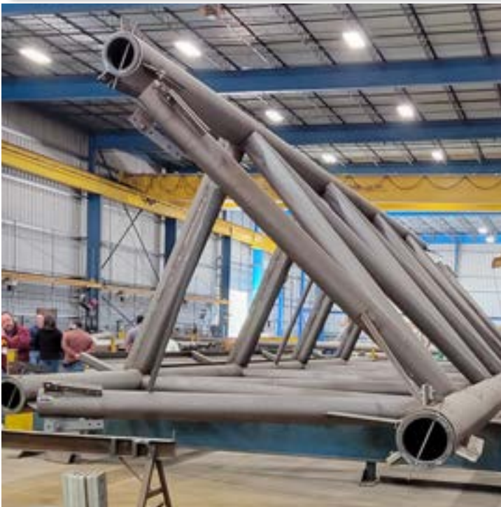
These trusses, being manufactured for the Charlotte Airport expansion shown below and to the right. The truss size dwarfs those standing next to it.
